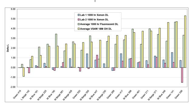
Figure 1 - 1000 Hour Xenon, 1000 Hour Fluorescent Average vs. VS4W 18 Months Ohio PVC Medium Blue, Green, and Beige Specimens
