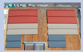
be used to predict the results of the outdoor protocol with a high degree of accuracy. Outdoor weathering tests were conducted in Florida, Arizona and northern temperate locations to obtain baseline data for comparison. This part of the research led to the development and subsequent publication of ASTM D6864.
