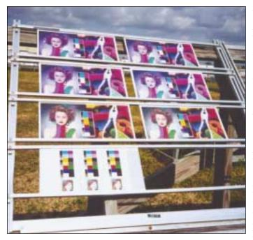
Figure 1. The appearance of photos may degrade over time due to bright indoor lighting or sunlight through window glass. These photos are being exposed outdoors at a test site in Florida to check for permanency.
